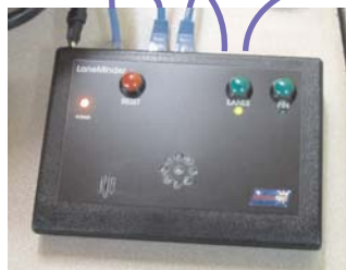
Control Module at Front Desk
